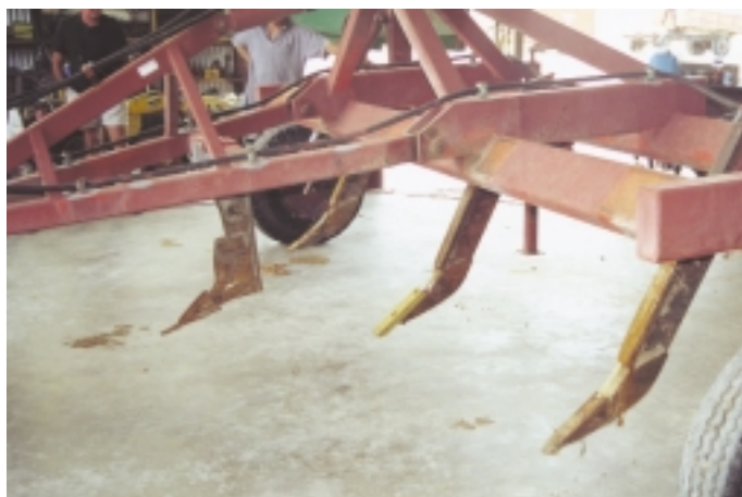
Delving tines can bring clay up from about 70 cm depth.
