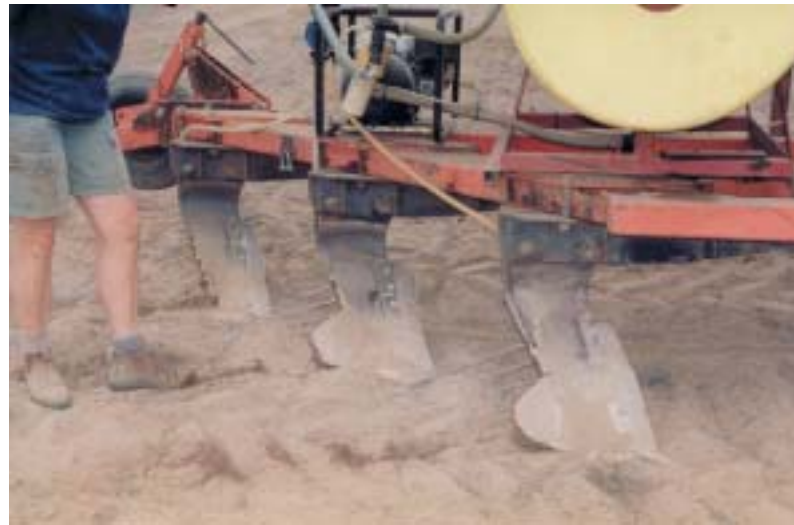
The paraplow is used to squirt liquid fertiliser to depth along the back of the blade —note the moisture.
