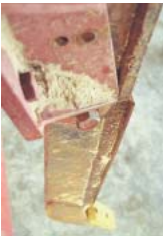
The delving tine up close —the leading edge is reinforced.
