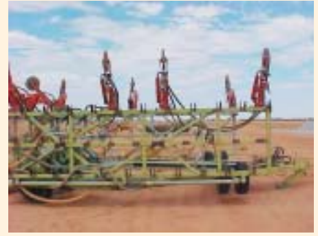
Summer crop seeder - an old Allfarm bar setup with ConservaPak tines on 1m single skip rows used for opportunistic seeding of fodder and grain sorghum.
