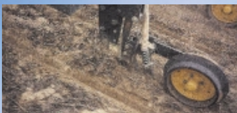
The Nichols opener can cultivate deep at the same time as sowing.
