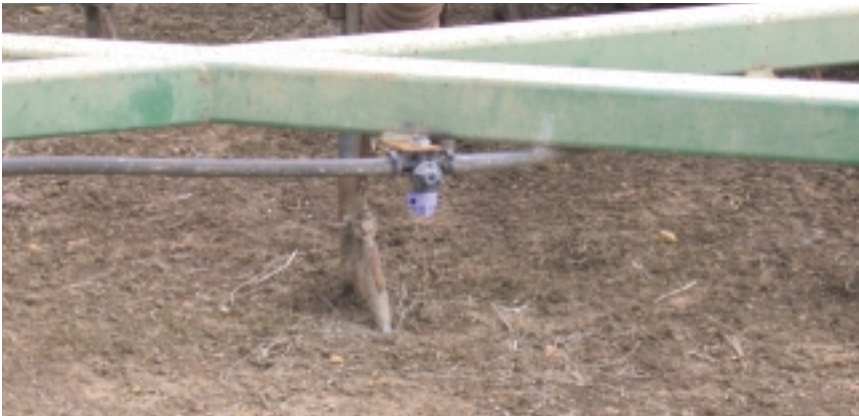
Nozzles mounted on the front of the seeder for timely trifluralin application.
