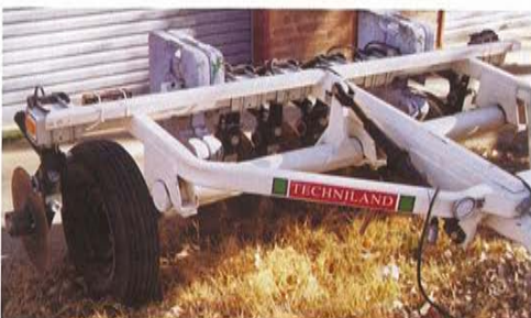
A salt sensing machine that can give electrical conductivity readings to 70cm depth—this could be useful to WA farmers. It is linked to a computer and can create a map of a paddock—knowledge is power! For more information see www.veristech.com .
