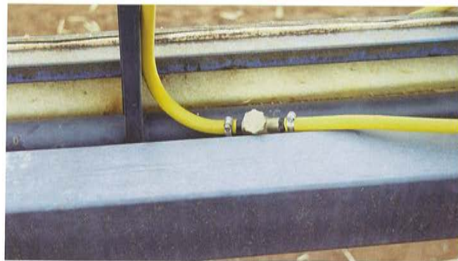
The needle valves can be clearly seen and likewise the mat with a few barley grass heads caught in it.
