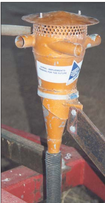
Gyrul air diffuser allows four inlets
