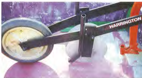
A simple paired row system for placing high rates of fertiliser safely near the seed and away from the weeds.
