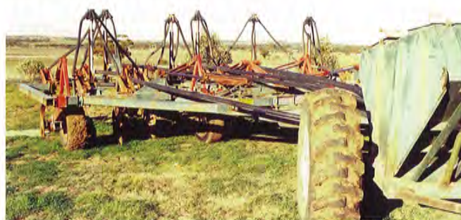
Richard made a seeder for no-till at a minimum cost. Note the black polypipes from seed bin to distributors.
