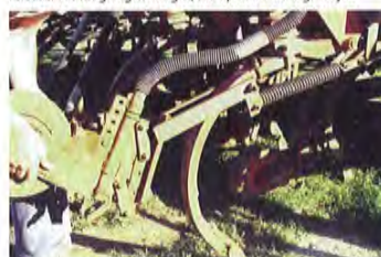
Below: Richard assembled a parallelogram opener with spring release. Although light-weight, the openers did a great job.
