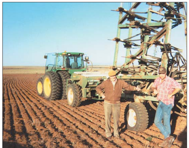
Geoff's father Felix and son Paul with Shearer Hydraulic Trashworker fitted with Harrington knives and split banding boots.
