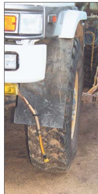
The nozzle located in front of the wheel puts out lots of water (has its own reservoir)—but it ensures good weed control in wheel tracks.
