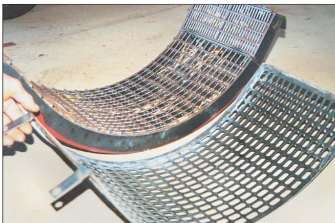
Below: Farmer designed plate (right) sits above the concave (left) and reduces canola seed loss.
