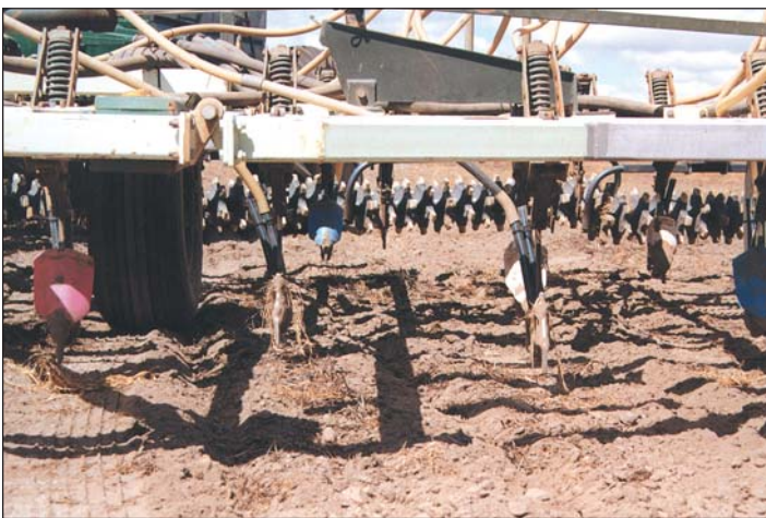
Geoffrey Marshall's seeder modified for wide rows. Two rows run close together to separate seed and fertiliser.
