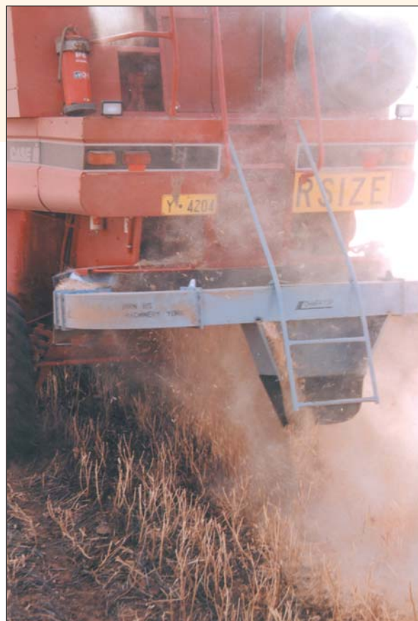
Chafftop in action, putting chaff on top of the header row.
