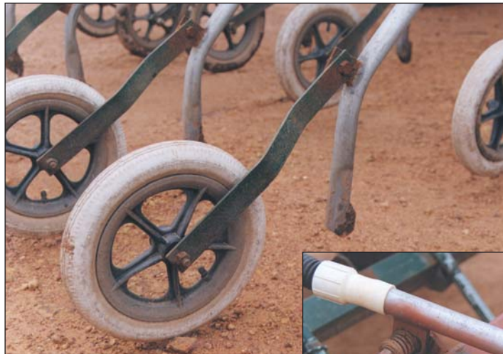
Above: Tony calls this seeding arm (copied from Graham Malcolm), a poor man's DBS. However, it is effective for Tony. Right: The top end of the seeding arm—fertiliser is placed ahead, in the bar behind a leading tine.
