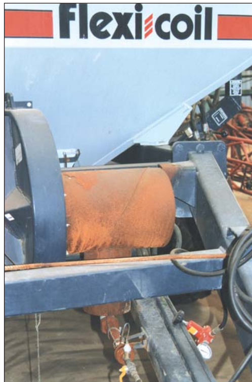
Rocks and thick chain are placed inside this 40 cm diameter drum and are heated from below with a propane flame
