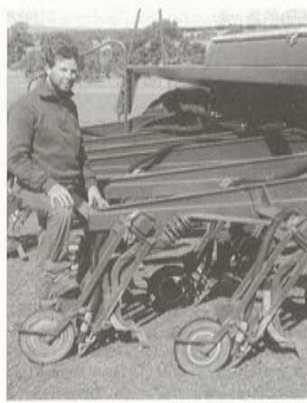
"Tine and parallelogram share common pivot point"
