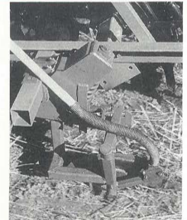
The Angled-Disc no-till opener developed by Canadian engineer Ben Dyck at ... Fabro Enterprises Limited, Box 517, Swift Current, Saskatchewan, S9H 3W3. Ph. (306) 778 3955, Fax (306) 778 3538
